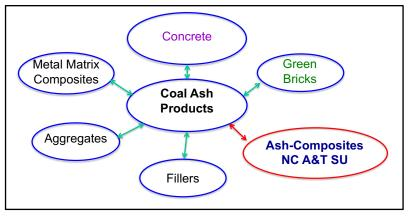
With introduction of Ash-Composite, we extended the use of coal ash to polymer-based particulate composites (see accompanying Chart). This composite is self-curing using the internal chemical energy, the foaming of the polymer helps to control the density and mechanical properties, the high percentage of ceramic particles makes the composite fire- and
